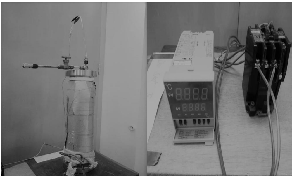
Fig. 1. (a)Torrefaction Reactor, (b) Electric Controller (Left) and Magnetic Contactor (Right)
